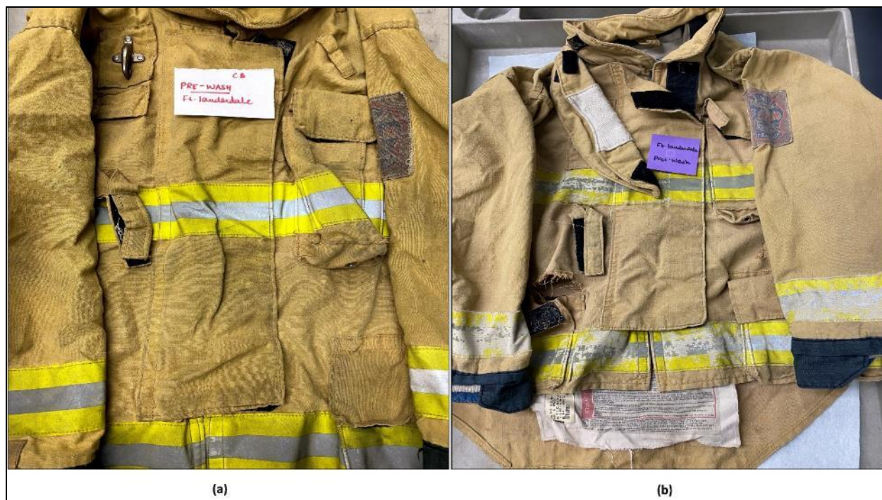
Figure 12-14: Effect of conventional wash on turnout suits (a)pre-wash (b)post-wash.
