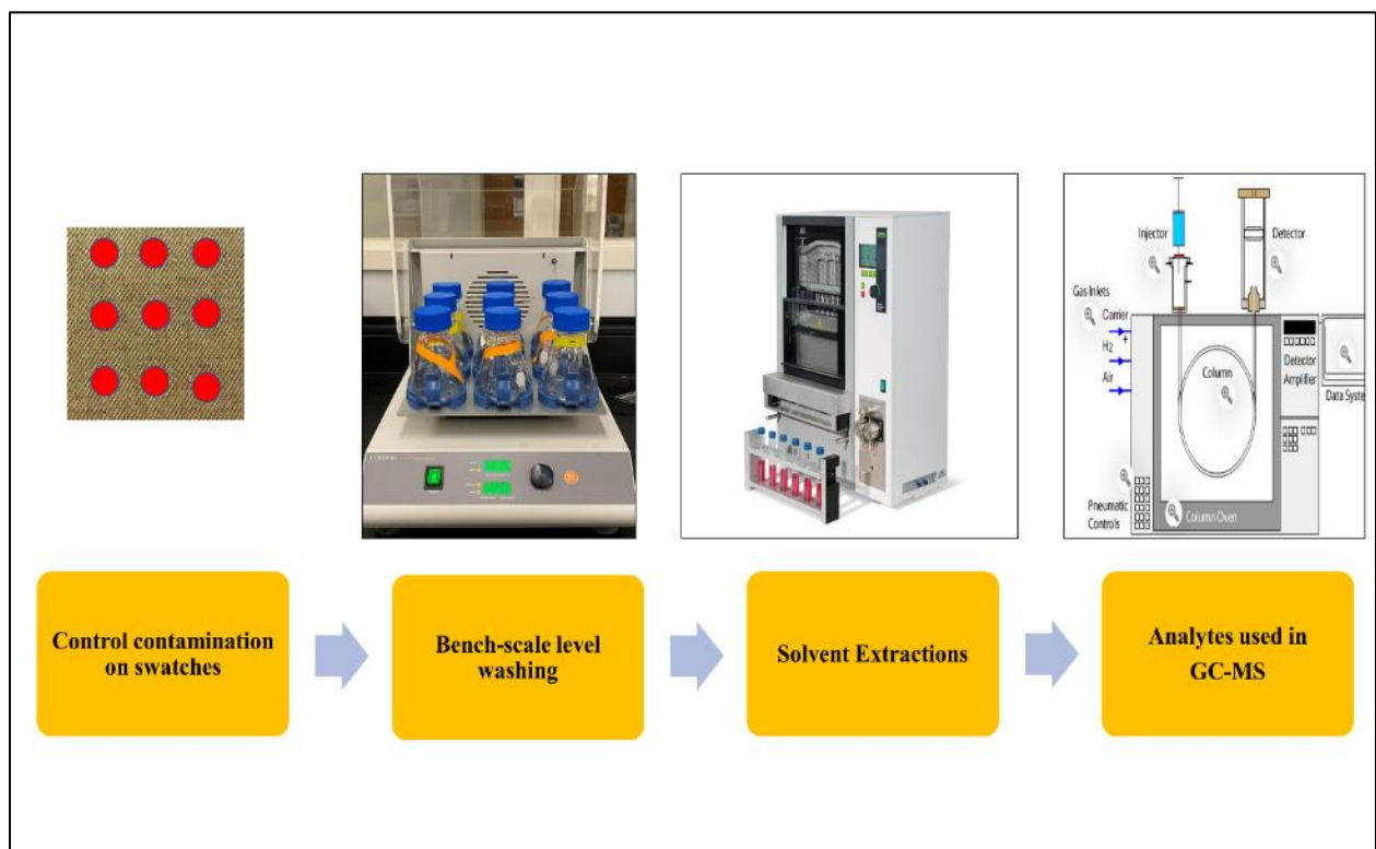
Figure 8-3: Process flow for bench-scale washing method.
