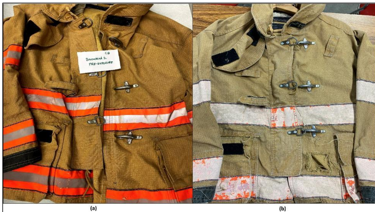
Figure 12-20: Effect of modified wash on turnout suits (a)pre-wash (b)post-wash.
