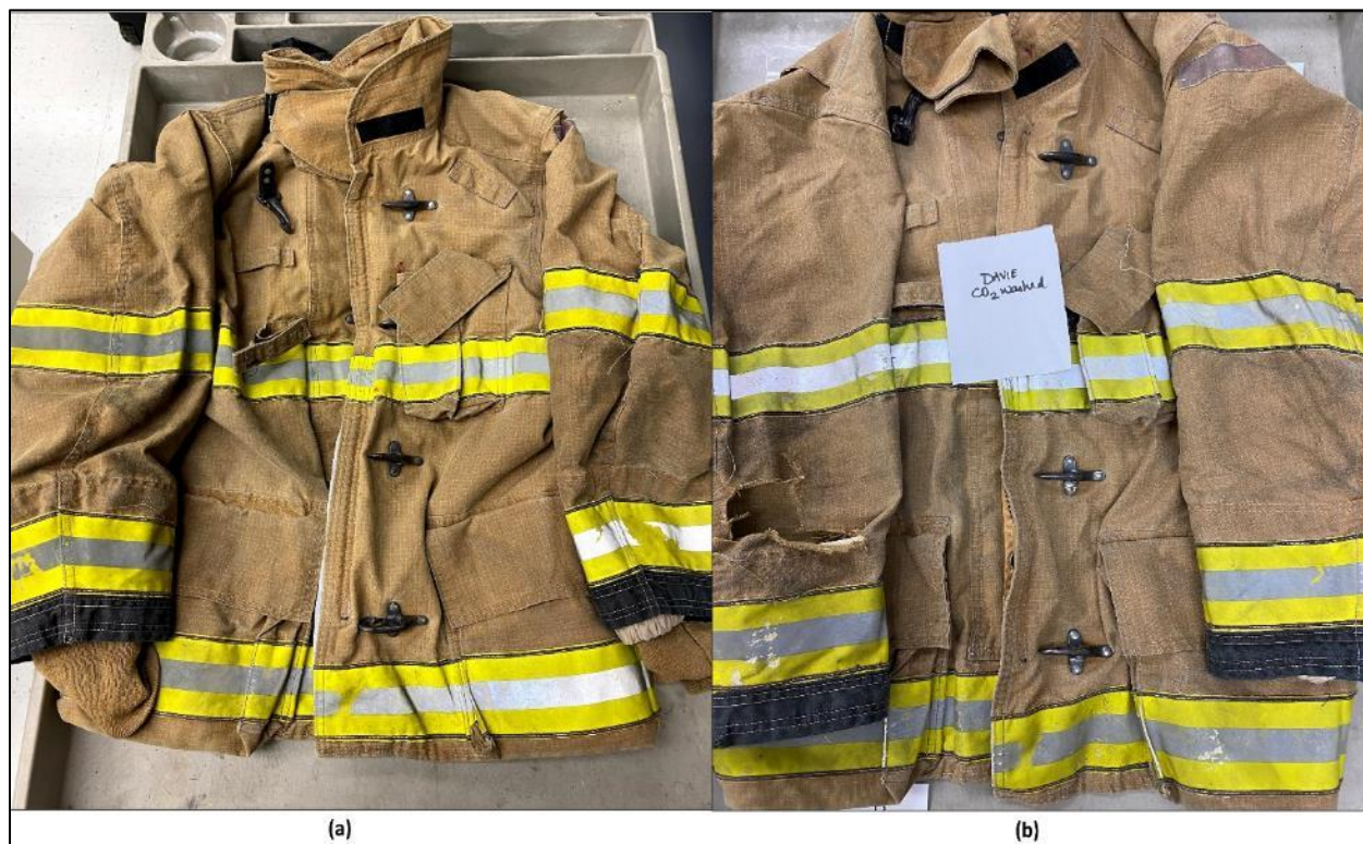
Figure 12-26: Effect of liquid CO 2 wash on turnout suits (a) pre-wash (b) post-wash.
